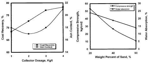
Fig. 1. Effect of collector dosage on the removal of coal fines from filter cake
