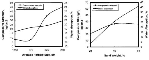
Fig. 3. Effect of particle size of sand on physical<br/>and mechanical properties of bricksFig. 4. Effect of weight percent of sand<br/>(for - 500 + 0 μm size fraction) on physical and<br/>mechanical properties of bricks
